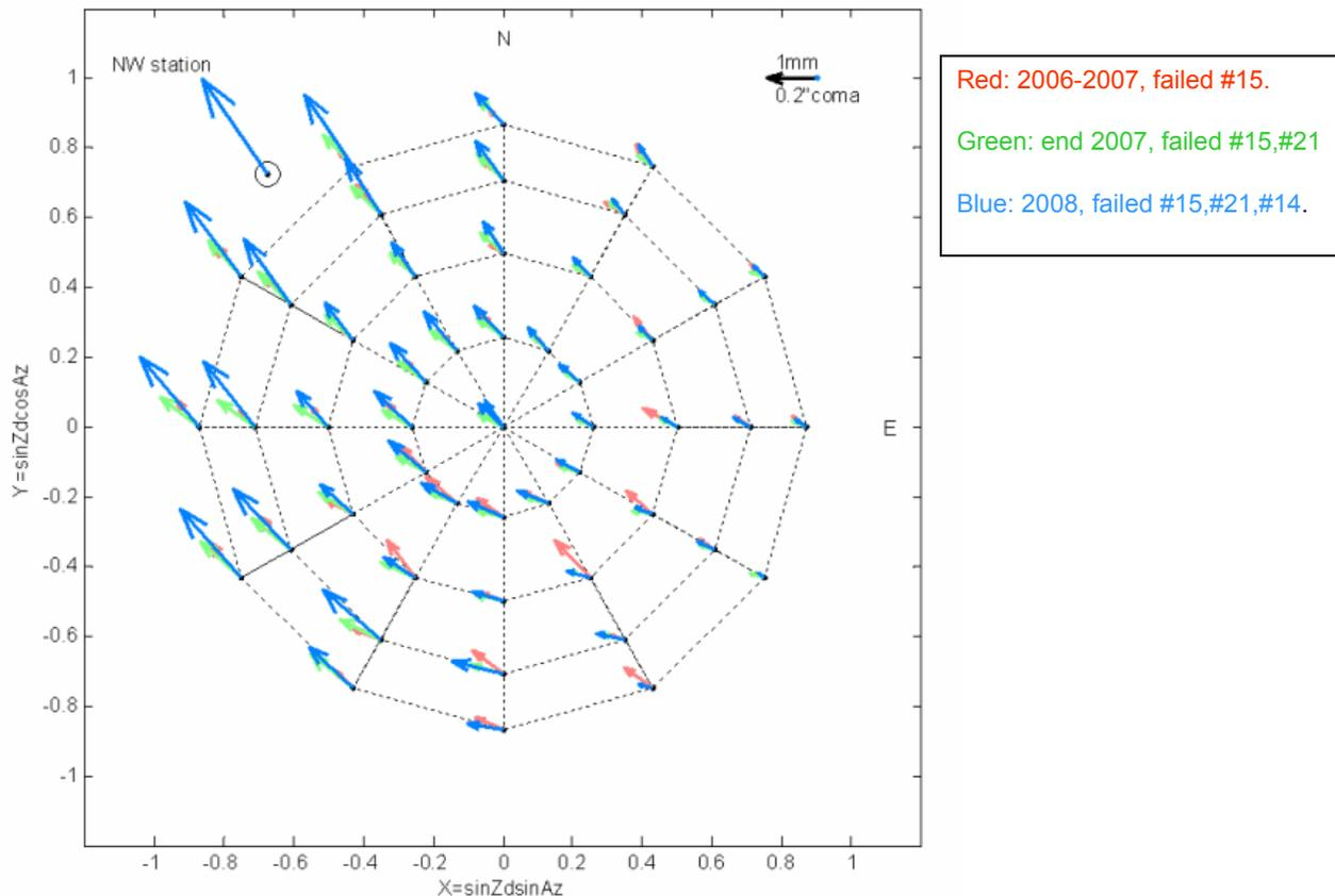
**Fig.1.** The Sky-map used to build the Blanco aberration correction look-up tables. The arrows represent the mirror displacement w/r to the cell as radial supports break.
