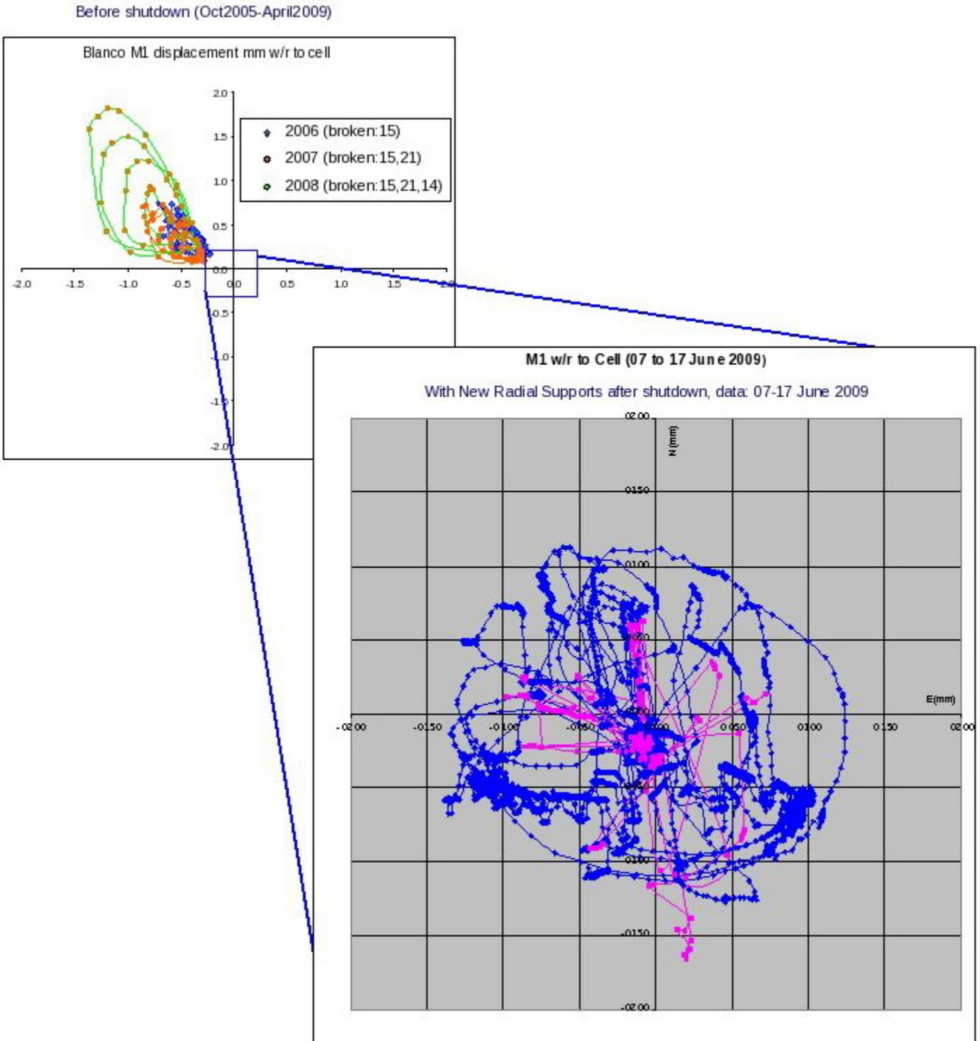
A Telemetry logging system was implemented (2) to keep track of the M1-related opto-mechanic Telescope parameters, like M1 radial displacement w/r to cell (Mitutoyos), axial hard-points load cells (Adam modules) and in the future, axial actuators voltages (Mamacs). Figure 3 are pictures of the Telemetry GUI showing the actual position of the Blanco main mirror in its cell during, roughly, the first week of May2010 (a) and the hard-points load in Kg at the time of the grab (b).
