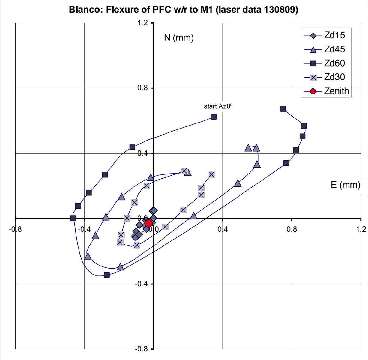
**Fig.4.**The Blanco top-ring displacement w/r to M.
