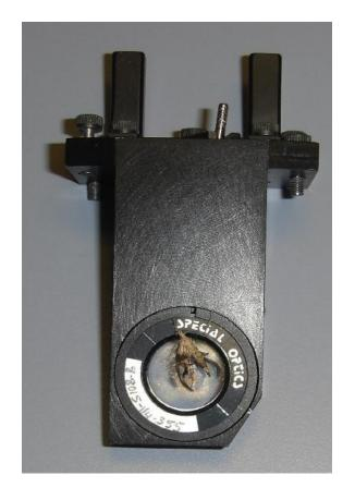
Protected LLT with thin-wire mesh It worked until... a smaller bug in October 2016 burned on M3!
