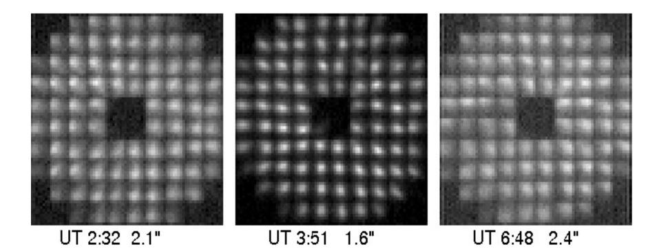
The spot size is determined mostly by the local seeing Now the 2x2 binning is used: less noise, faster
