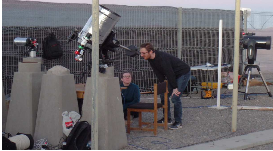
Figure 2: Portable turbulence profilers: RINGSS (left), SHIMM (center), and FASS (right, on the tripod).
