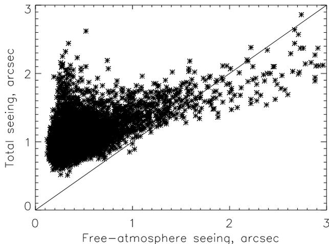
Figure 1: Seeing measured by MASS and DIMM at Cerro Pachón in January 2003.
