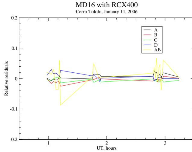
Figure 5: Residuals of scintillation indices obtained during first tests of MD16 with the Meade RCX400 telescope.
