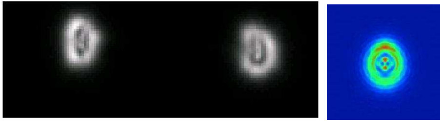
Figure 2: Defocused spots showing astigmatism in the DIMM channel with wrong orientation of L1. Left: tests with the MASS-DIMM, right – Zemax modeling of this effect as an intra-focal image.
