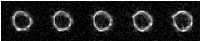
Fig. 5. Five consecutive ring images distorted by turbulence and detector noise. Each image is 16x16 pixels (13.8''), the average ring radius is 3'', the interval between images is 3 ms, the wind speed is 10 m/s.
