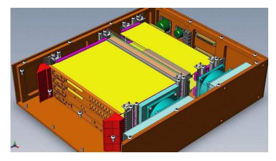
Figure 3: Monsoon Orange conceptual drawing. Box size 435x390x108 mm, mass 9.9 kg.
