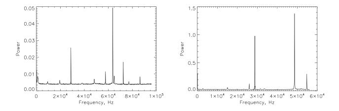
Figure 6: Power spectrum of the CCD line signal in the fast (left) and normal (right) readout modes obtained on Dec 30, 2009 at the telescope.
