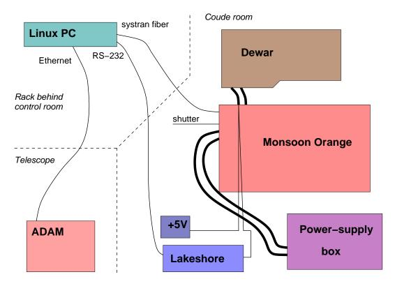
Figure 2: Elements of the new controller system and their connections.
