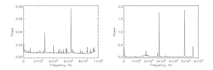
Figure 5: Power spectrum of the CCD line signal in the fast (left) and normal (right) readout modes obtained on Dec 29, 2009 in the lab.
