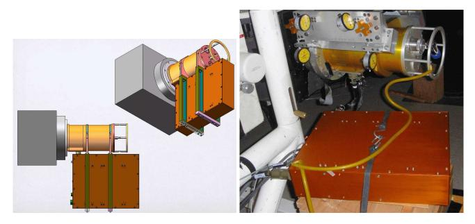
Figure 9: Left: design of the Monsoon Orange mechanical coupling to the dewar (implemented, but not used). Right: provisional installation of the Monsoon Orange on Dec 30, 2009.
