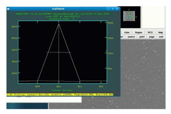
Figure 7: Illustration of the CTE evaluation.
