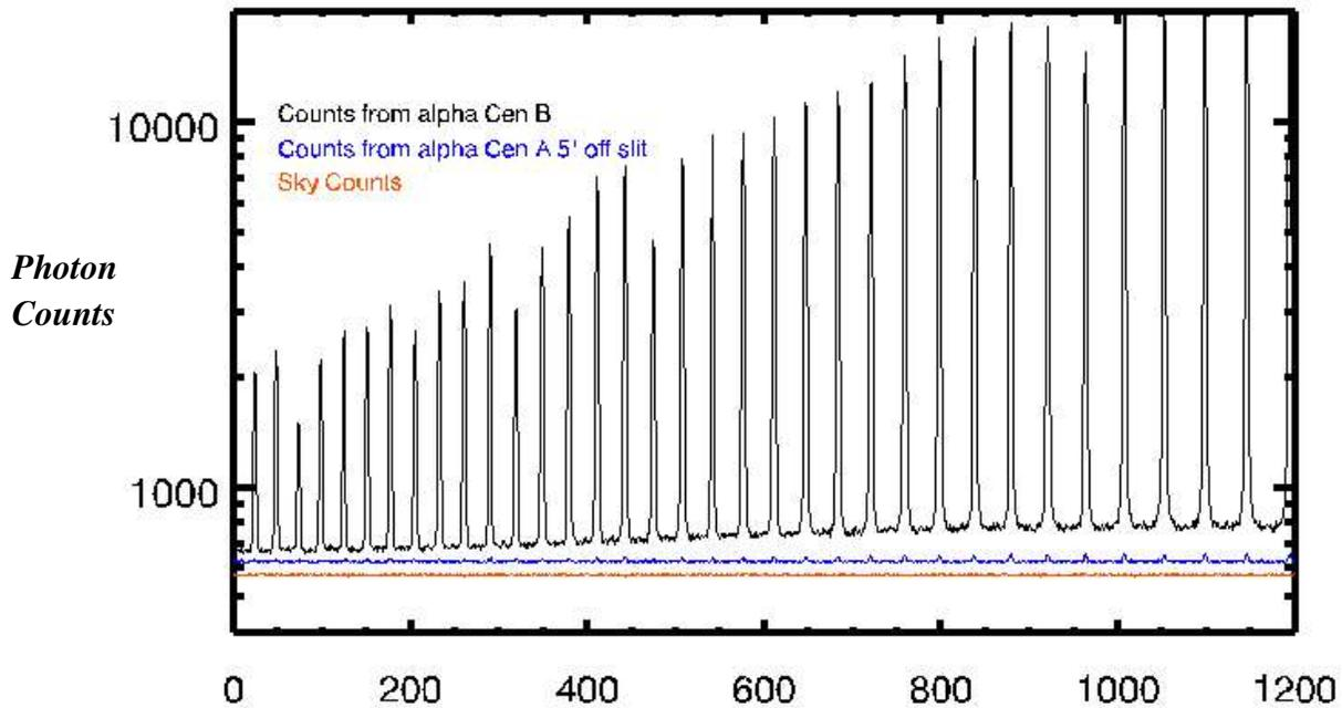
**Figure 2.** Column count of flux from a 20 second exposure of alpha Cen B, a 2 minute exposure of alpha Cen A when placed 5 arcseconds from the slit and a 2 minute sky exposure. The light spill-over from alpha Cen A is only 20 dN, suggesting it will contribute about 1 part in 30000 to the alpha Cen B counts (this should have no impact on the Doppler observations).
