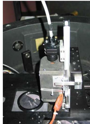
The iodine cell was built at SFSU and shipped to CTIO a few weeks before the observing run began and was installed in a housing that rotates into place between the optical fiber and the entrance slit to the spectrometer (in the close-up figure on the right; the red cord connects to the temperature controller).
