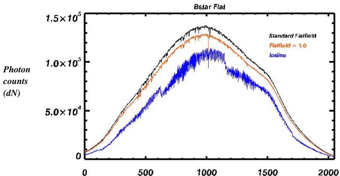
*Figure 3. Extraction of one order of an observation of a bright Bstar. The top plot (black) is taken with the standard, normalized flatfield. The red curve is offset by 0.95, but extracted with a uniform flatfield of 1.0 and shows the same functional shape, perhaps a combination of the blaze function and some loss of flux on the red side of the chip (beyond about 1500 pixels). The blue curve shows an observation of the Bstar through the iodine cell, with the expected absorption line depth.*
