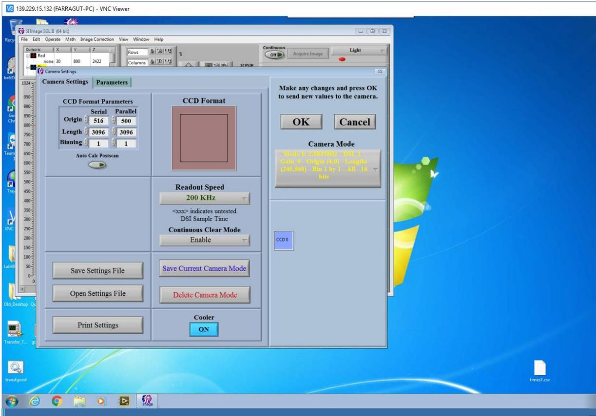
10. From the SI Image front panel, open the Camera Status window to display the current CCD Temperature and Pressure. The operating Temperature and Pressure of the Blue Camera are -106.5 C and 0.000 Torr. Log the Temperature and Pressure
