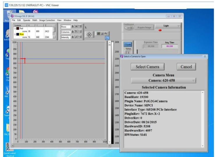
7. Check that the Cooler is ON as indicated in the image below. If it is OFF, Click OK and open the Camera Status Panel. The pressure should be 0 or  $\sim < 0.001$  Torr ( $\sim 10^{-3}$  Torr or 1 mTorr), see image below. If not, the Goodman cryostat (camera) needs pumping, which is done by the SOAR day crew, and usually requires a full day or so. **WARNING: DO NOT START COOLING THE CAMERA IF THE VACUUM HAS NOT BEEN REACHED.**
