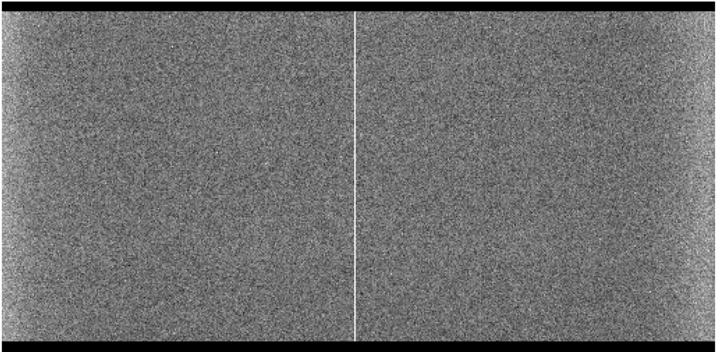
Figure 1. Combined Bias frames in Spectroscopic 1x1 mode (average of 20 individual bias taken with the 200ATTN0 readout mode).
