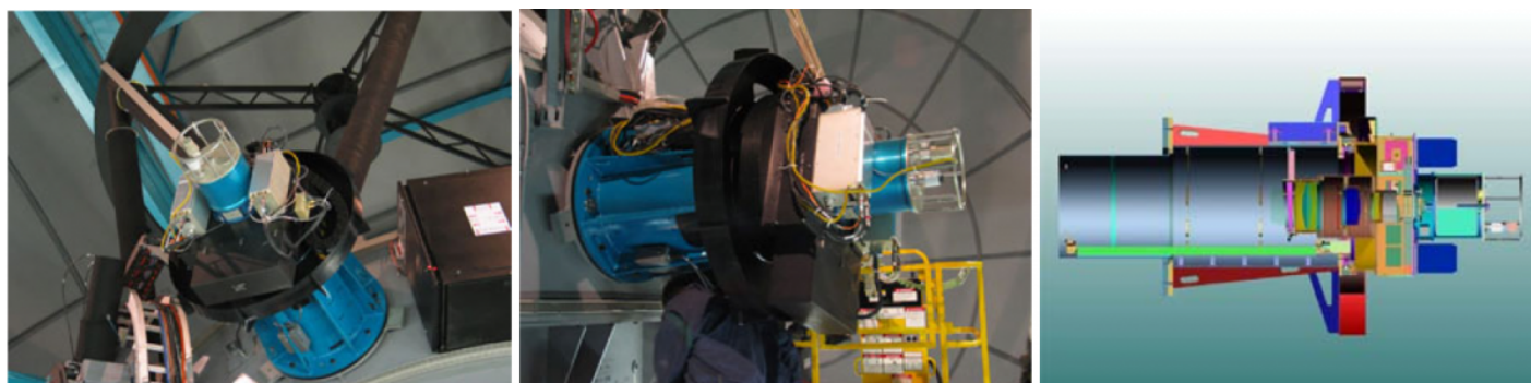
Figure 1: Two views of the SOI mounted at one of the bent Cassegrain foci of the SOAR telescope. The smaller blue cylinder is the CCD mosaic dewar and is flanked by the two rectangular Leach controllers, the round black part is the cable wrap, and the large blue tube bolted onto the telescope is the main body of the instrument holding the linear ADC prisms, one of which can move over a distance of nearly one meter. The drawing shows the basic lay-out of the instrument in a cut-out view. From left to right the light encounters: ADC prisms, optics module, two filter slides, the shutter, and finally the CCD mosaic.
