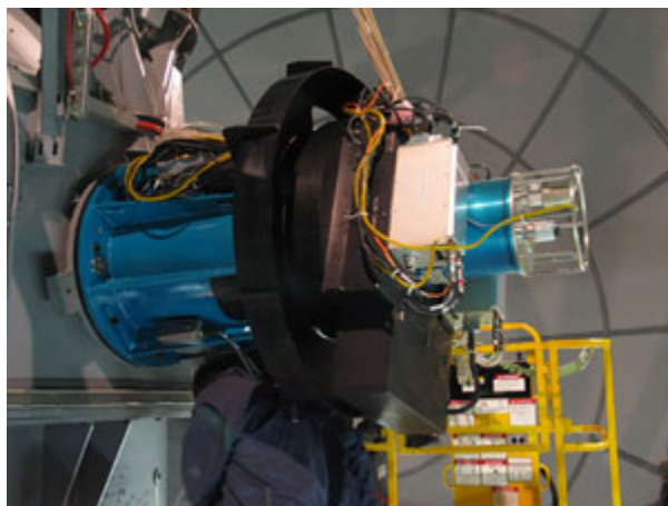
Figure 4: The SOI system mounted on one of the bent-Cassegrain foci of the SOAR Telescope. The dewar containing the 2 CCDs is the smaller blue cylinder located on the right. The SDSU Leach controller is the silver box located in front of the dewar.
