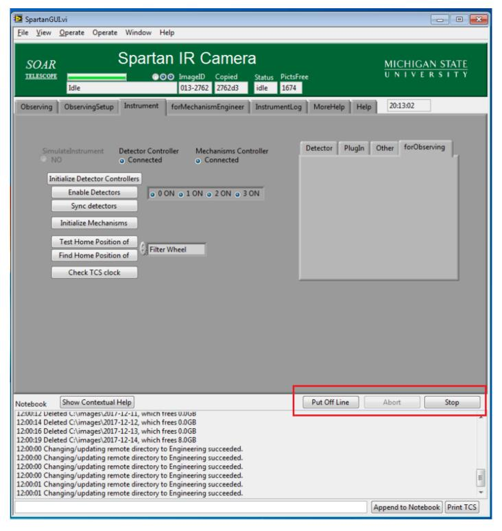
**NOTE -** it is possible to stop the GUI, for example by clicking inadvertently on the red "X" on the upper right. The instrument status will show "stopped" instead of "idle". The "run" arrow (see above) should be visible; click on it and the GUI should recover. You will likely also need to click the "run" arrow for the scripting interface (TUI).
