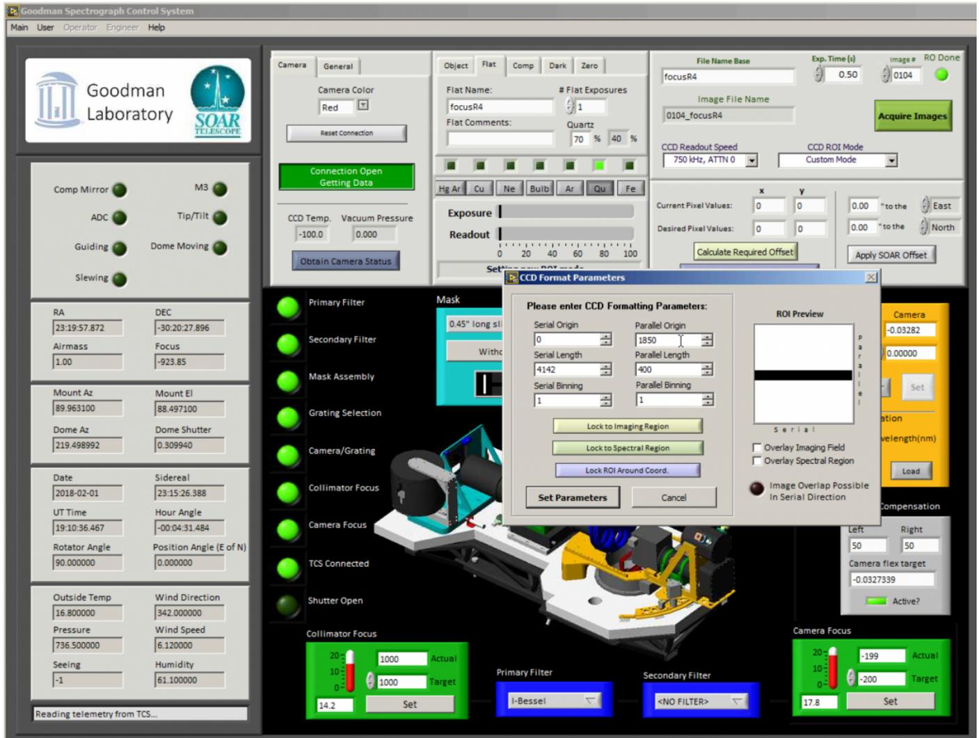
Figure 2: Change the ROI mode for faster readout (you can use a more 'vertical' geometry for this case)
