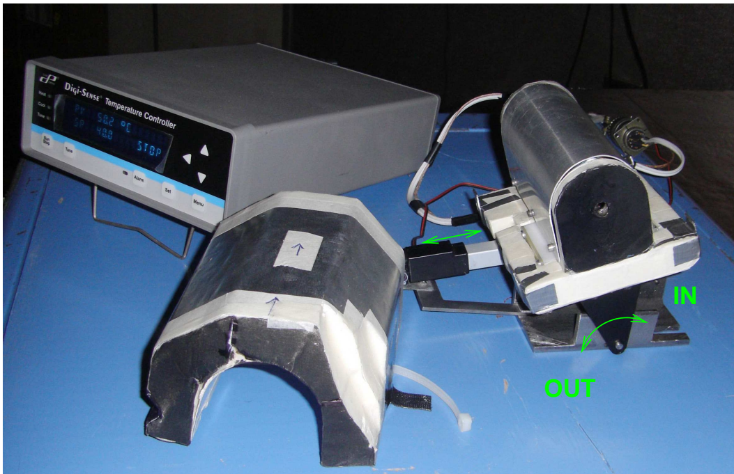
Figure 21: Photograph of the iodine cell container and its actuation mechanism. Part of the thermal insulation is removed. The Cole-Parmer temperature controller is in the background.
