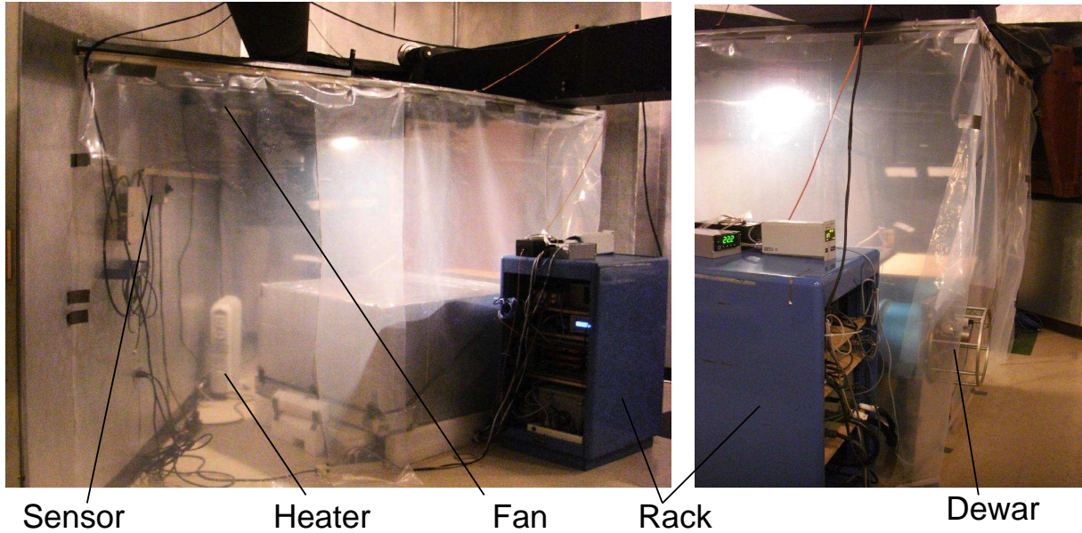
Figure 25: Pictures of the plastic curtain around CHIRON (“warm room”) and elements of its temperature stabilization. The electronic rack and N2 exhaust from the dewar are outside the controlled environment.
