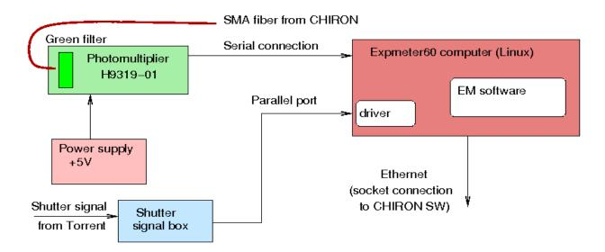
Figure 1. Block-diagram of EM hardware and connections.
