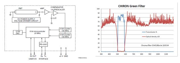
Figure 2. Block-diagram of the PMT circuits (left) and the transmission of the filter (right).
