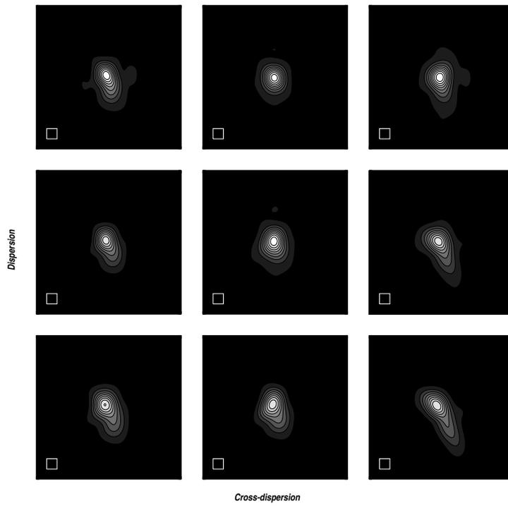
Figure 9: Average PSF per CCD region when the detector is in focus.
