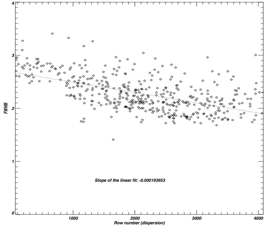
Figure 4: FWHM of ThAr as a function of row number (dispersion direction).
