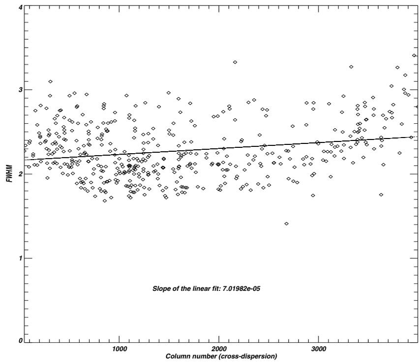
Figure 5: FWHM of ThAr as a function of column number (cross-dispersion direction).
