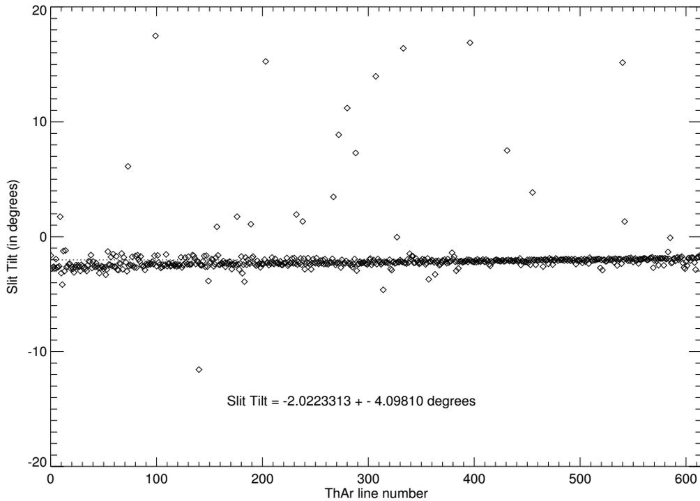
Figure 8: Measured slit tilt for all identified Th-Ar spectral lines after correction.
