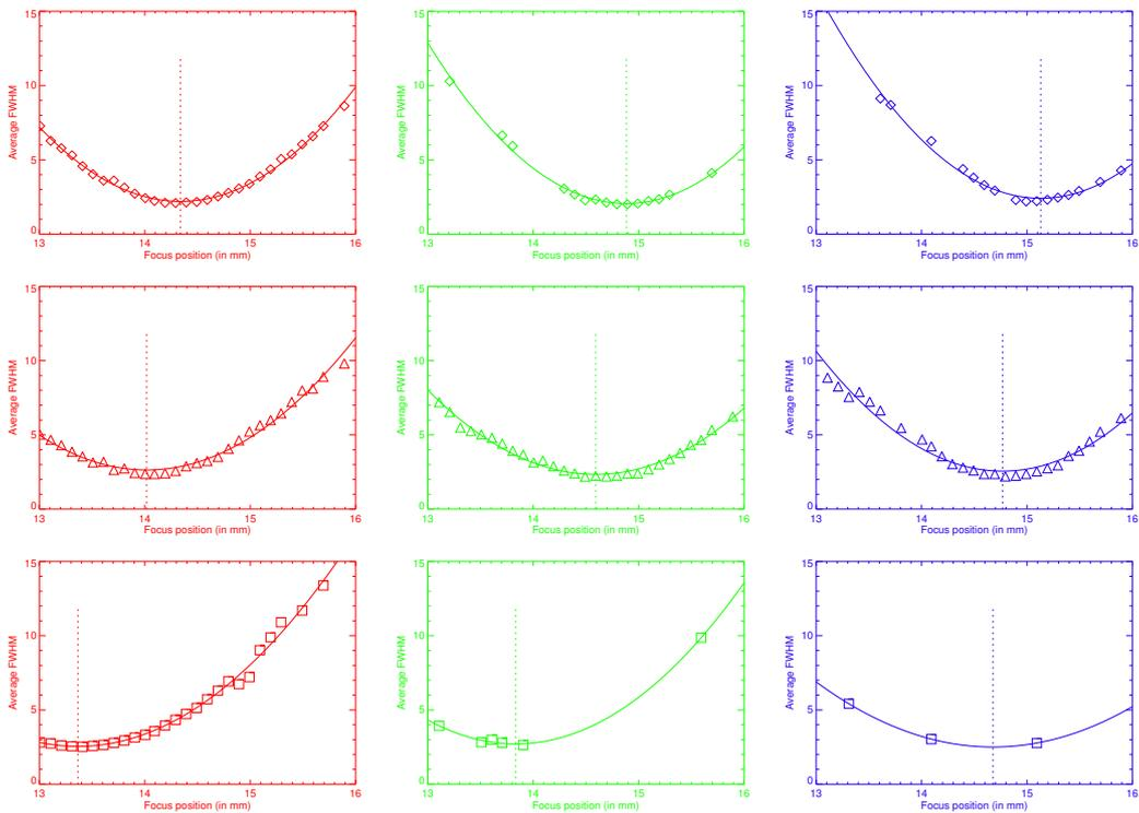
Figure 1: Through-focus average FWHM of ThAr lines per region of the CCD before adjusting the CCD tilt.
