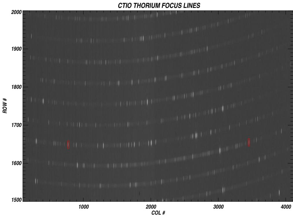
Figure 6: This figure illustrates how we have corrected the CCD rotation. Two spectral lines, on two adjacent orders, symmetric with respect to the center of the CCD and corresponding to the same wavelength must fall on the same row.
