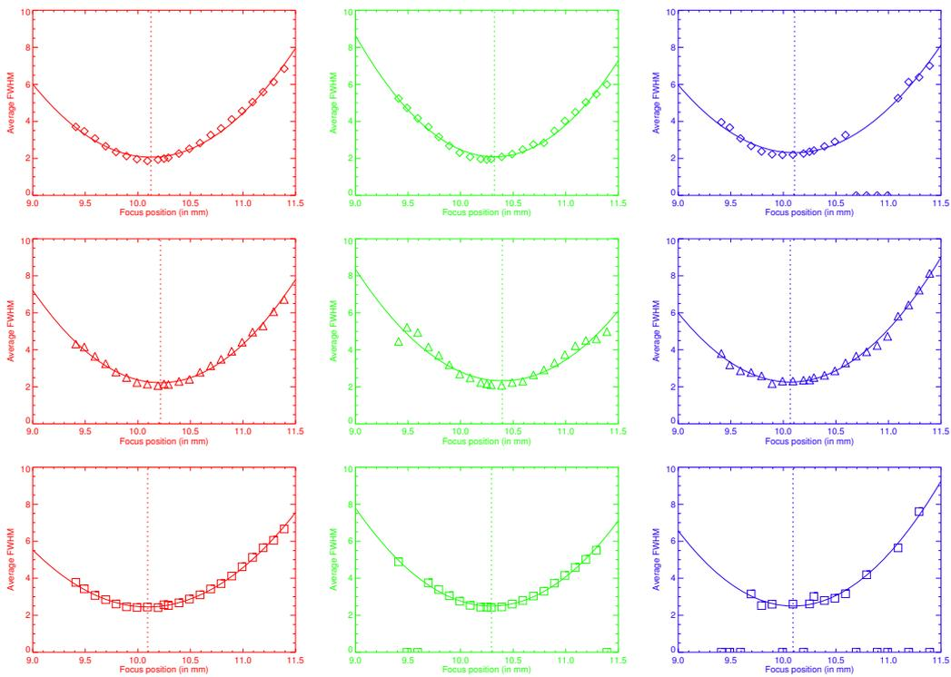
Figure 2: Through-focus average FWHM of ThAr lines per region of the CCD after adjusting the CCD tilt.
