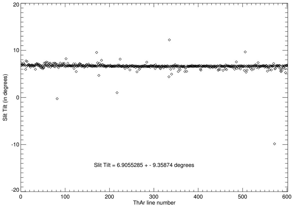
Figure 7: Measured slit tilt for all identified Th-Ar spectral lines before correction.
