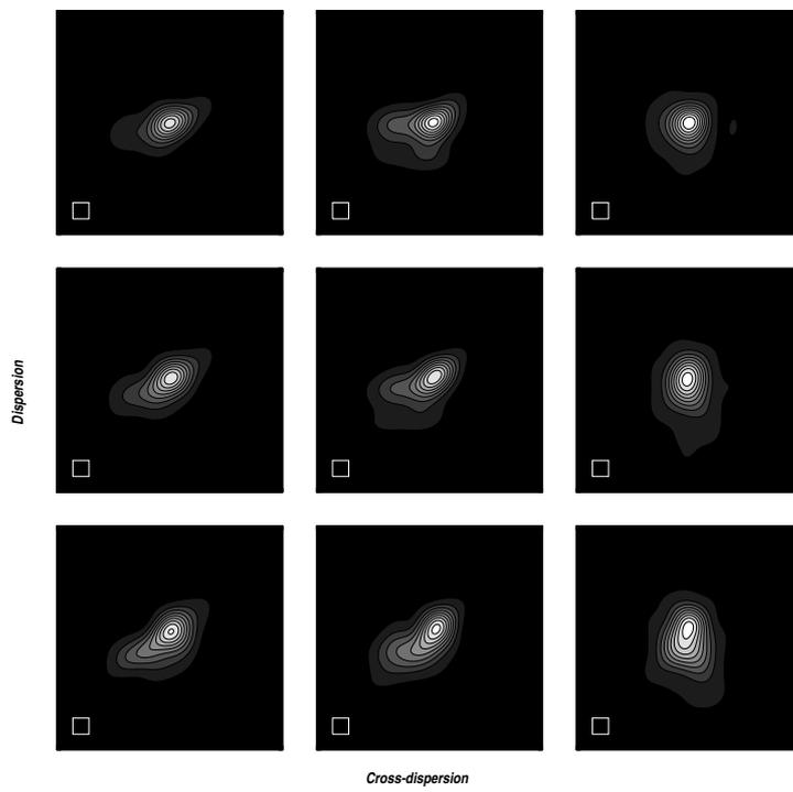
Figure 11: Average PSF per CCD region when the detector is 0.5 mm extra-focus.
