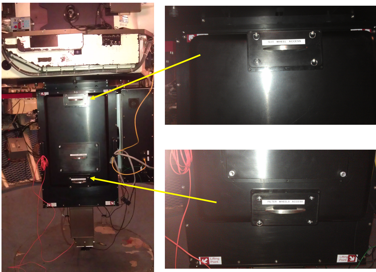
Figure 32: Location of access ports for slits (top) and filters (bottom).
