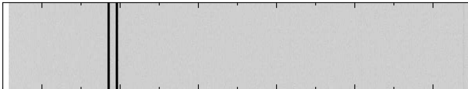
HgAr Penray – COSMOS Red Grating Center Slit
