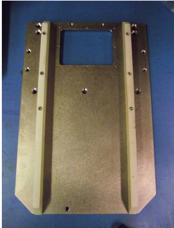
Step 3.1 Base plate showing rail orientation
