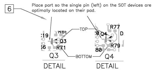
Use a bare wire, 26-30 awg, to connect from the side with 2 leads (right) to the closet vias. Top pin to nearest top via, bottom pin to nearest bottom via.
