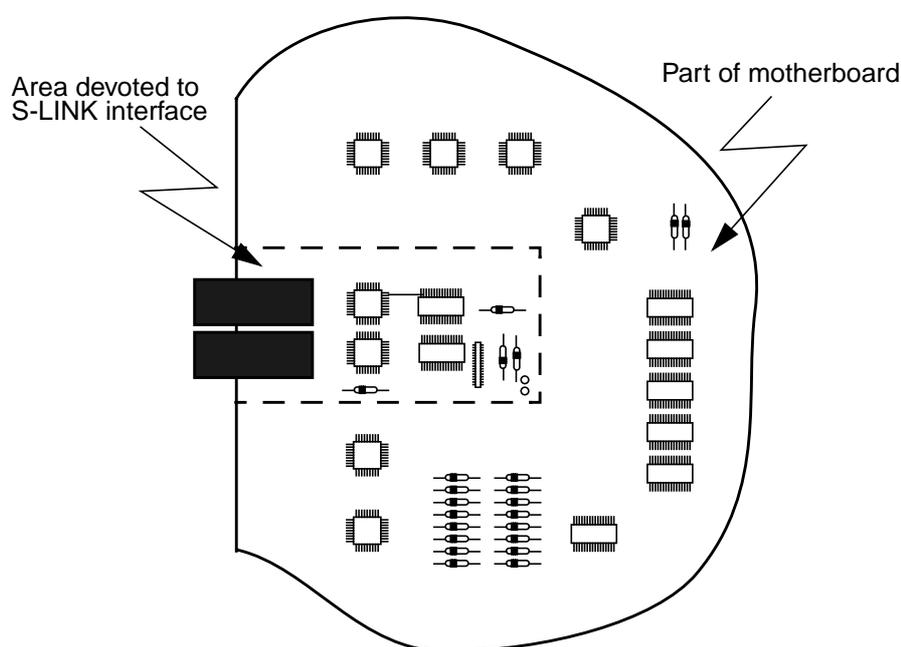
Alternatively, some users may wish to have separate S-LINK cards which are then mounted on the motherboard. If such users have no preferred physical arrangement, it is *recommended* that they construct the S-LINK cards according to the description given in Section 5.2.
