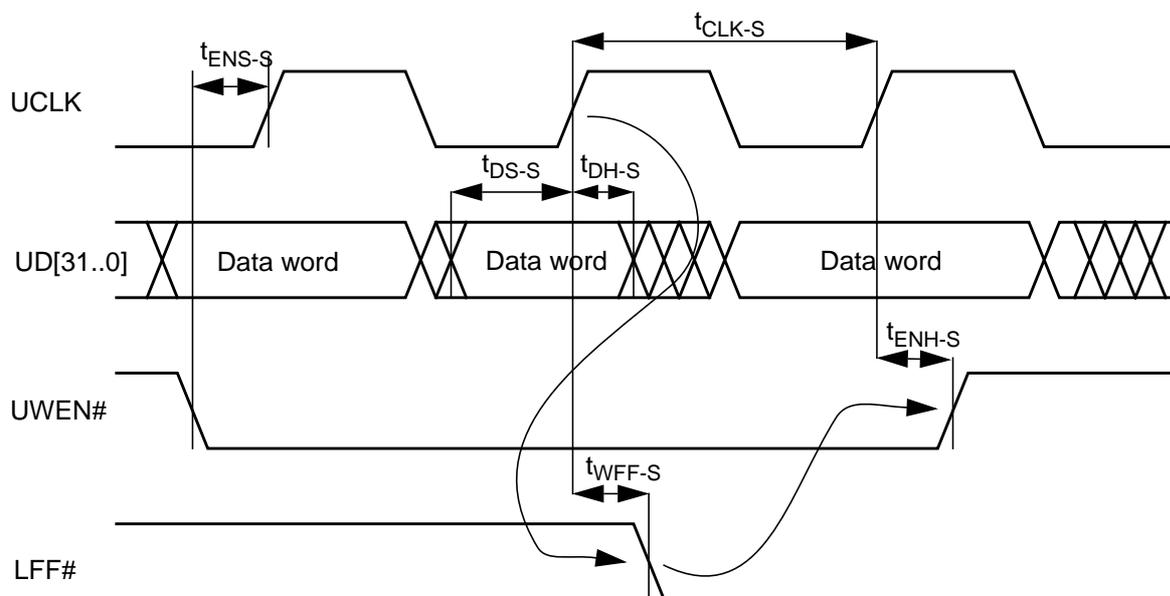
Note: In this diagram, only one extra data word is transferred after LFF# goes low. In fact, up to two words may be transferred.
