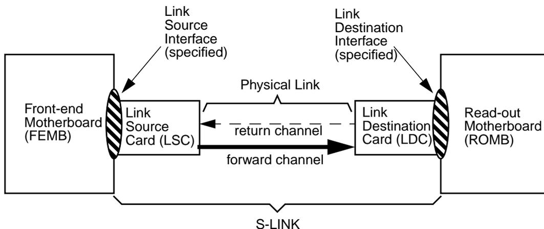
In many applications a uni-directional data channel will be required. In other cases the user might require to send flow control and other information back to the FEMB. The S-LINK, therefore, can be constructed in either a *simplex* or a *duplex* version.
