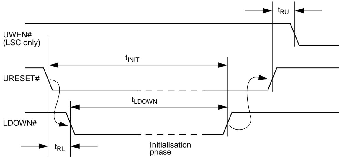
**TABLE 12.** Reset Cycle Timing Parameters
