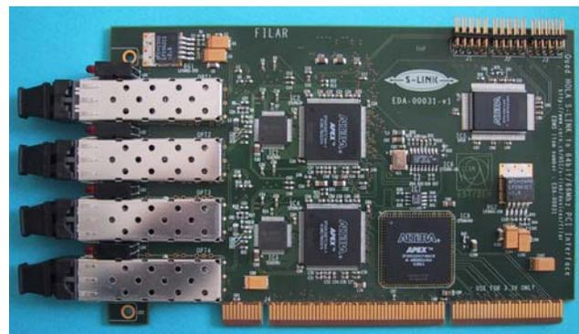
Figure 1: Picture of the FILAR PCI interface card
