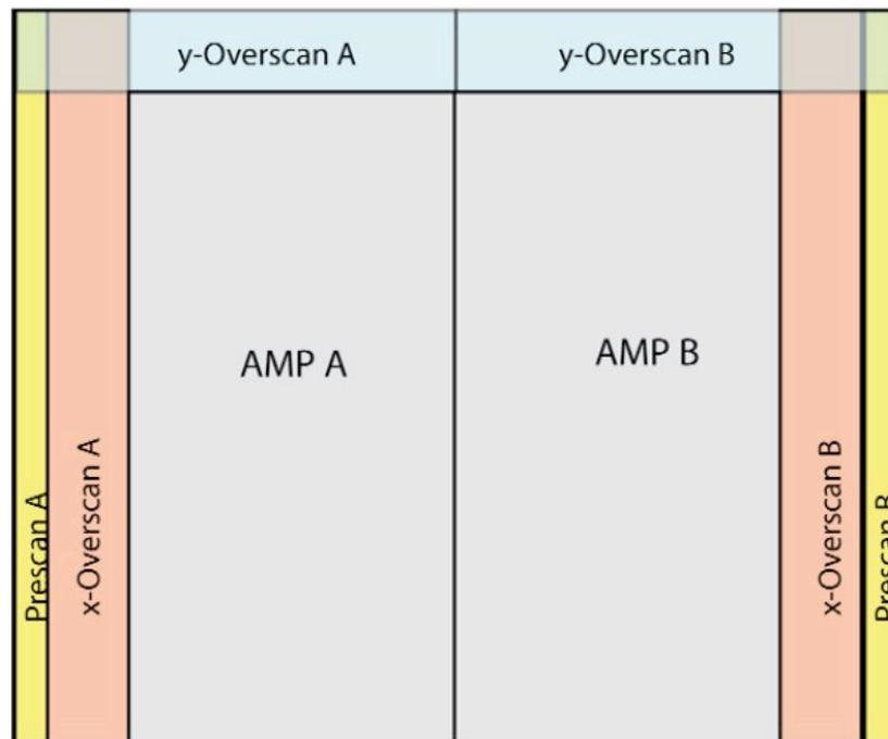
Figure 2.3: Schematic of the image array just after read-out of DECam. Note that there is some overlap in the pre-scan and overscan regions. (DES 4809-v3)
