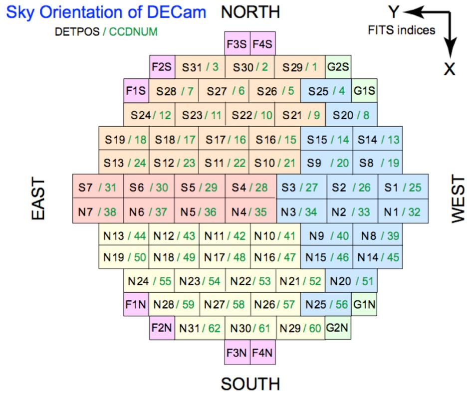
Figure 2.2: Orientations on the sky and spatial footprint of the FPA for DECam. 2k x 2k CCDs labeled as “F” will be used for focus and alignment control; those labeled as “G” will be used for guiding. Two amplifiers on each chip may be used for parallel read-out. The pixel coordinate origin is in the lower-left corner of each detector array.
