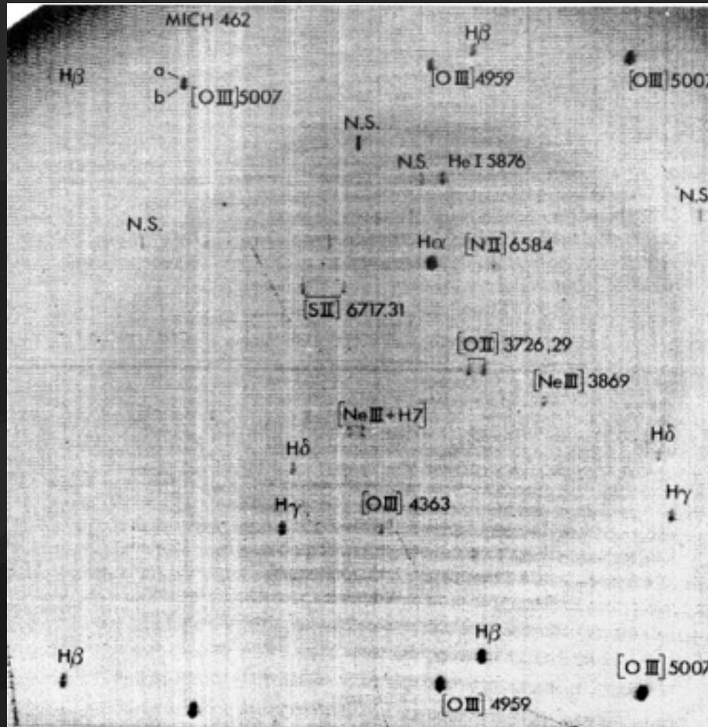
Melnick+ 1988: SIT-Vidicon Echelle spectrograph at CTIO 4m telescope
